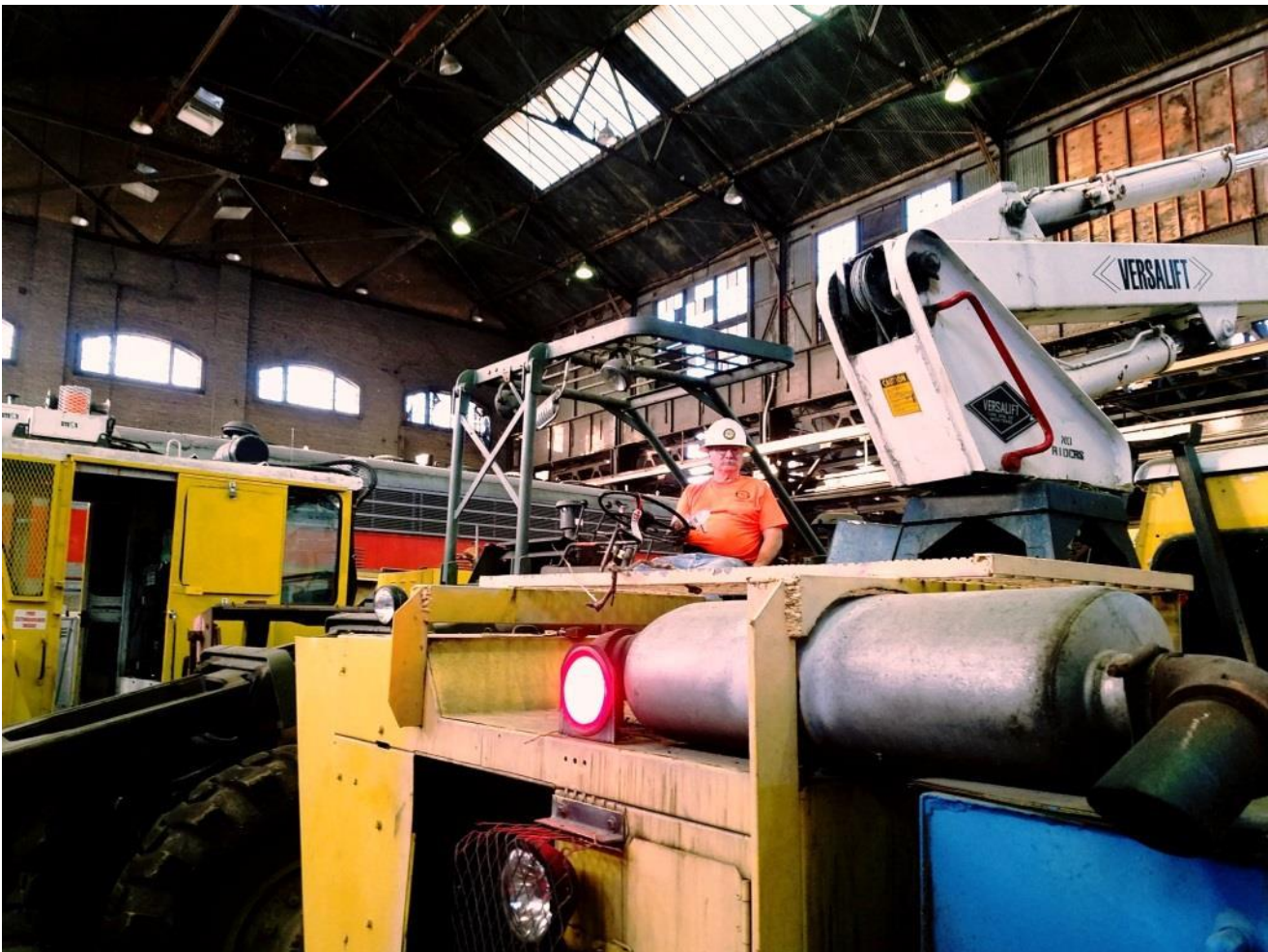
Mike Harris checks out the tilt controls after he cleaned and repaired the hydraulic valve
